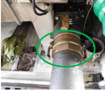
Securing the recovery arm
