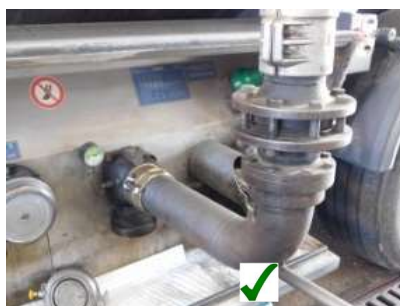
Connection of recovery arm
