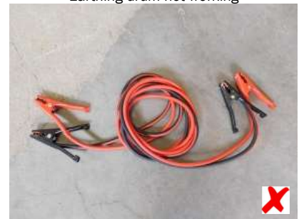
Use of jumper cables
