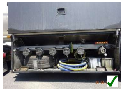
Storage of spare wheel and hose by the manufacturer
